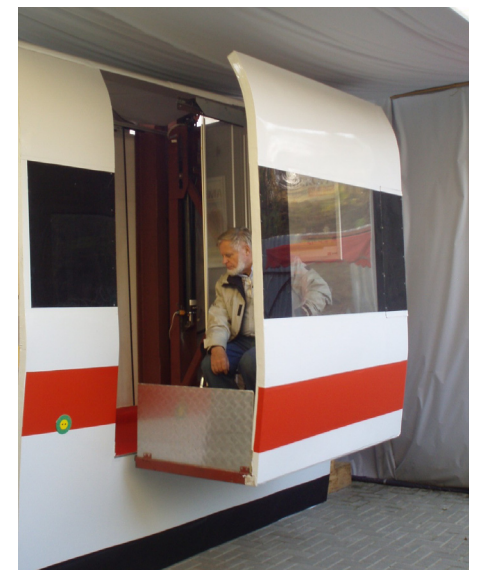
Cabin hoisting lift for the “long-distance and high-speed trains”
